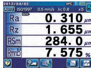
4-parameter display: four parameter measurement results
