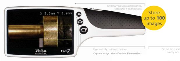
Suitable for production environments, CamZ provides high resolution magnification (up to 14x) and documentation, where you want, when you want.
