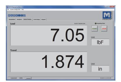
View real time load and travel readings on an enlarged simulated instrument display.
