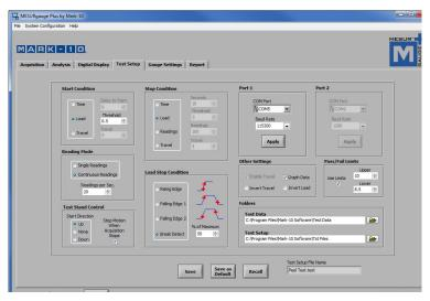
Configure test start and stop conditions.
