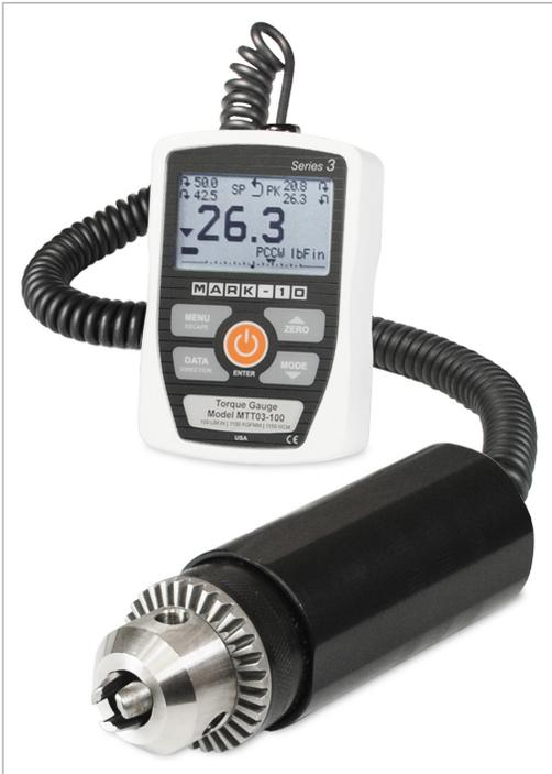
Series TT03 digital torque gauges are designed for clockwise and counter-clockwise torque testing applications in virtually every industry, with capacities from 10 ozFin to 100 lbFin (7 to 1,150 Ncm). A dedicated remote torque sensor with Jacobs chuck can be used to grip a sample, bit, or fixture. The gauges' rugged aluminum housing allows for hand-held use or test stand mounting for more sophisticated testing requirements.
